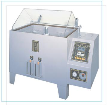
Salt water spray test device: This device is used to test the surface treatment of various materials. The so-called treatments include coating, electroplating, films of organic and non-organic materials, anodizing, anti-rest oil and corrosion resistant treatment, which may achieve the purpose of keeping the items from being corroded for a longer period.
