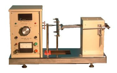
The GWT-200 Test Set incorporates a control unit, a traverse unit and the glow wire, all mounted on a robust base plate. The traverse unit is so arranged that the specimen carriage is mounted at the same level as the glow wire and this considerably reduces the contamination of the carriage from residues resulting from the testing. Suitable stops and a carriage retainer are built in to ensure that the actual testing can be carried out with the minimum of inconvenience.
