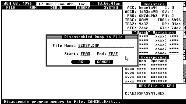
Figure 11: Disassemble Memory to a File.
